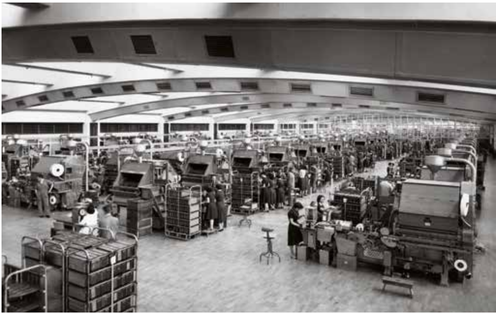
Making: cigarettes are placed on trolleys and moved to drying
