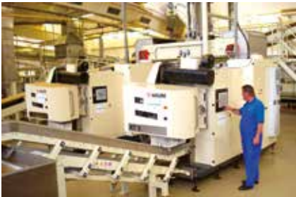
Top: EVA high temperature dryer Bottom: David Bell operating a new Hauni tobacco leaf-cutting machine
